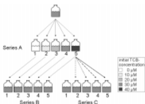
Figure 1. Experimental setup to test for growth linked to reductive dechlorination of TCB. Each bottle depicted in series A, B and C represents a triplicate of cultures. The series B cultures were inoculated with 0.5 ml of the various series A cultures. Series C cultures were inoculated with 0, 0.125, 0.25, 0.375, or 0.5 ml of a series A culture grown on 40 \mu M TCB.
